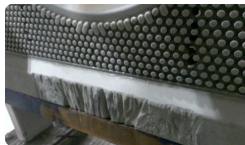
Figure 1 - Plate seal edge wear
