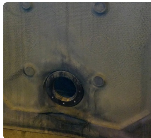
Figure 1 - Plate seal edge wear
