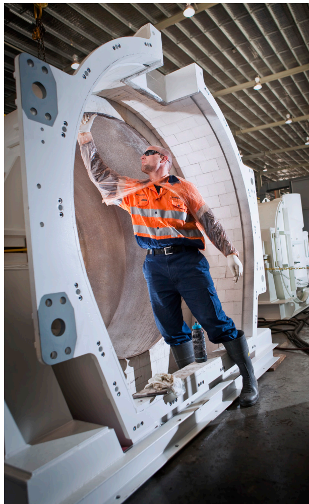
Applying WEAR MAX to centrifuge housing
