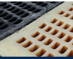
FLS screen media optimisation replaces rubber with polyurethane and increases productivity screen-deck-media\_polyurethane\_case-study.pdf (flsmidth.com)
