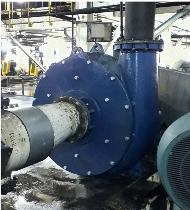
Our gravelMAX™ pump in a heavy media cyclone feed application in coal processing
