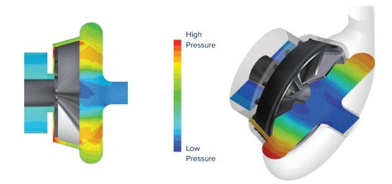
Recessed impeller creates a vortex that agitates slurry around the suction to keep solids in suspension
