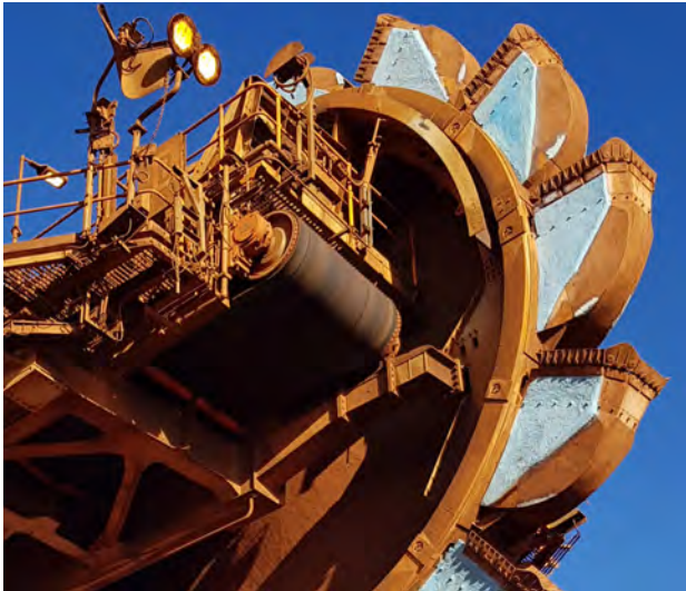
WEAR MAX® applied on reclaimer bucket wear surfaces
