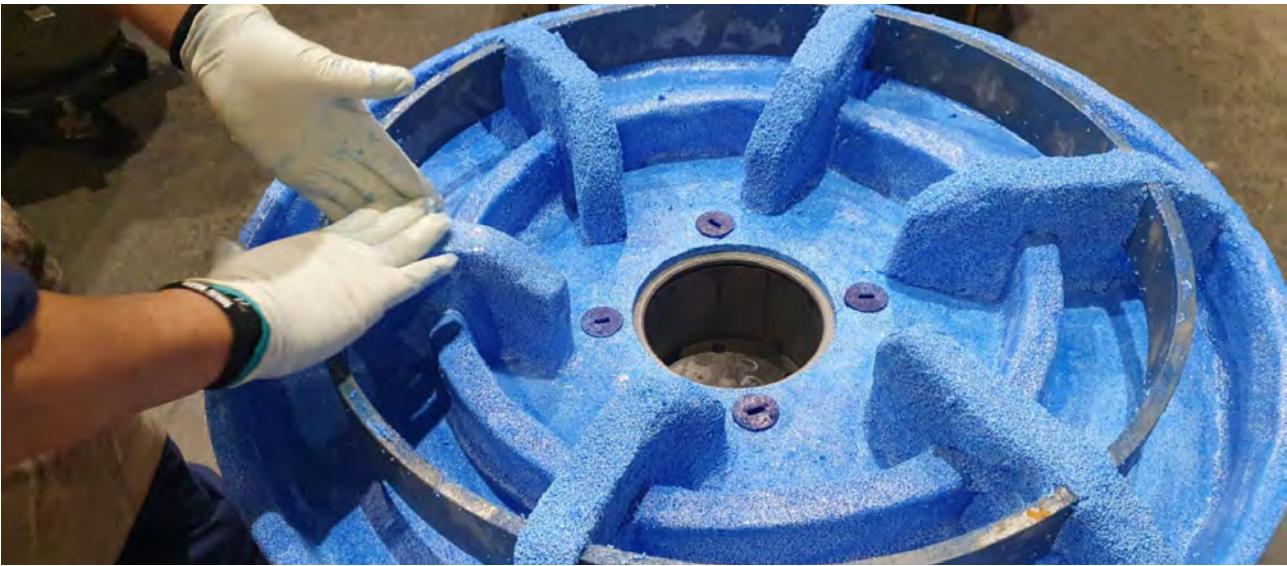
WEAR MAX® is applied to all wear surfaces of centrifuge feed distributor
