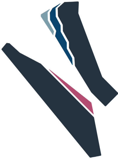
Typical configurations of bowl and mantle arrangements for maintaining product consistency as liners wear.
