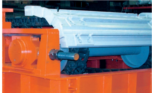
Tail shaft of apron feeder RKF 3.0 x 8.3 - D10.
