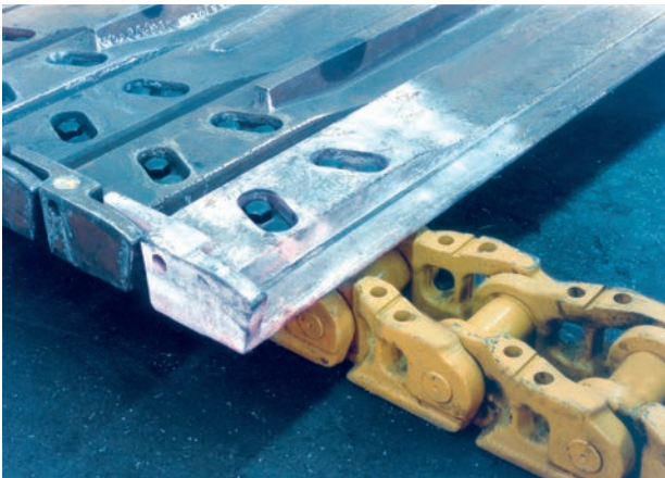
Cast aprons checked for surface cracks.
