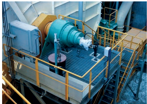
Hydraulic drive with axial piston motor.
