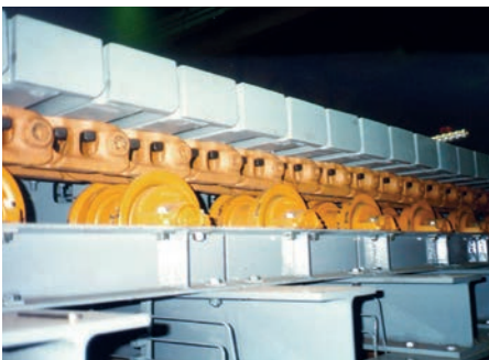
Apron feeder RKF 2.2 x 15.8 - D8 with inboard chain.
