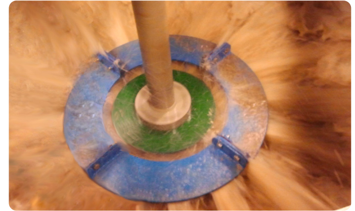
Wide flow jets produced by the nextSTEP rotor and the cross pattern from the patented slotted nextSTEP stator increase the chances of flotation
