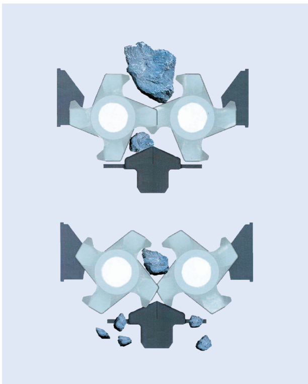
Crushing principle of the CenterSizer with breaker bar
